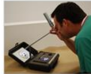
Check illumination at distal tip
