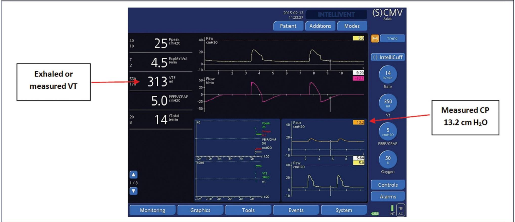
FIGURE 3 – Time Stamp 11:23 AM, Elapsed Time 59 Minutes / Exhaled VT = 313 mL and CP = 13.2 cm H 2 O.
