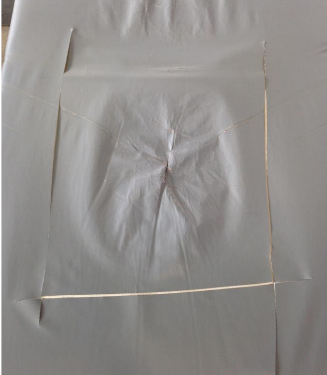
Mattress with obvious cracking and staining: Removed from service and the cover cut away...
